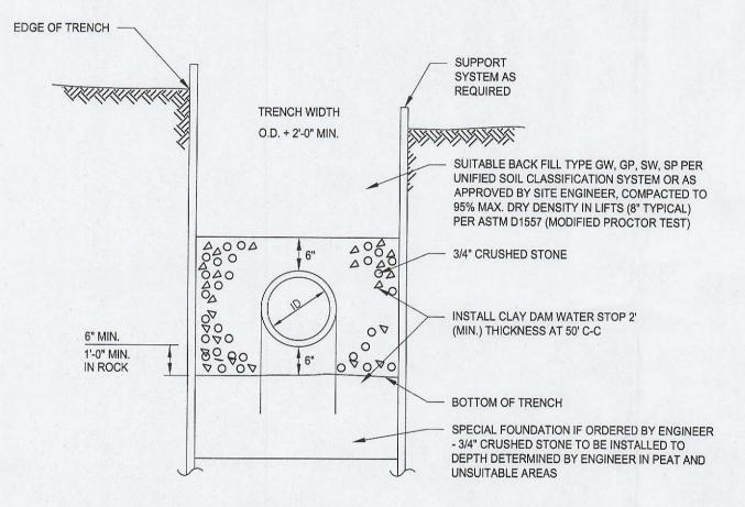
TYPICAL SANITARY SEWER TRENCH SECTION
