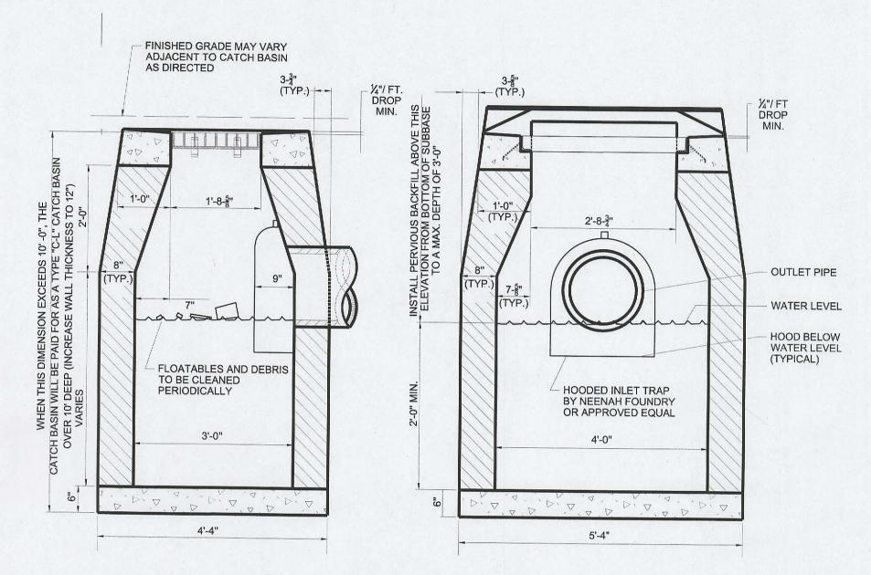
TYPE "C-L" CATCH BASIN WITH HOODED INLET TRAP
